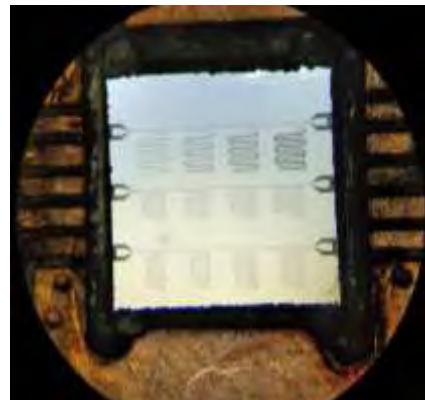
Figure 1: SC Al/Sapphire resonators designed with different surface participation ratios
