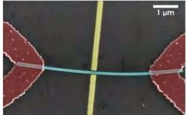
Figure 1: SEM image of the gated superconducting device.
