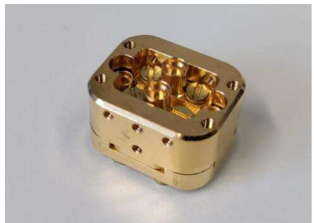
Figure 2: Photograph of a travelling wave parametric amplifier in a connectorized microwave package. The dimensions are 17.7 mm x 21.7 mm x 13.4 mm.
