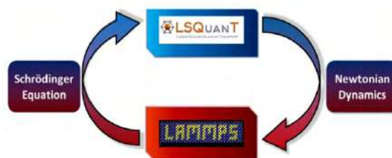
Figure 1. Schematic of the self-consistency cycle for the atomistic simulation of coupled charge and ion dynamics.
